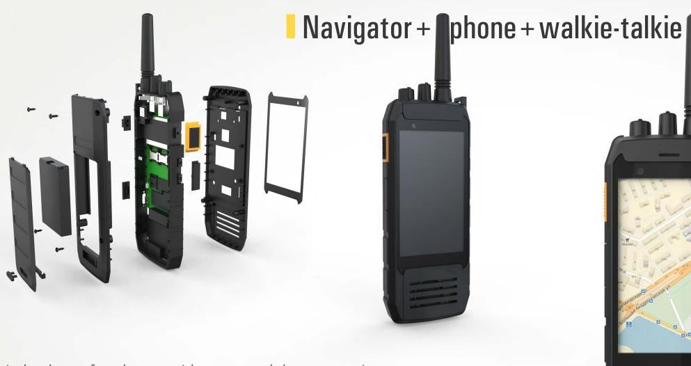
A shockproof enclosure with water and dust protection.
