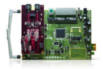
Our engineers designed a subscriber router for providing voice over IP services in broadband networks. This platform can be used for rapid development of network devices with VoIP features + interfaces: FXS, GbE, USB 2.0, and WiFi 802.11b/g/n.
