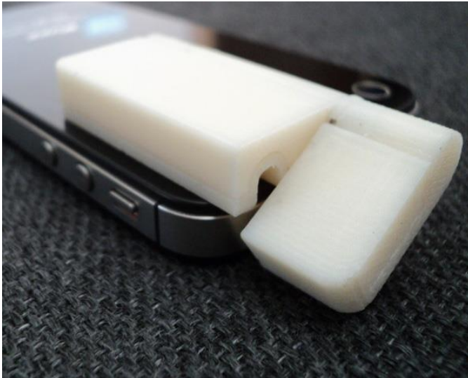
Figure 5. DO-RA.uni enclosure prototypes constructed in a 3D printer
