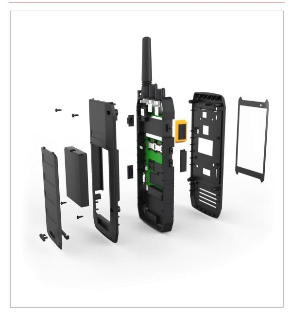
At the final stage of the project, we made a prototype of the enclosure using FDM technology and tested it for assembliability.
